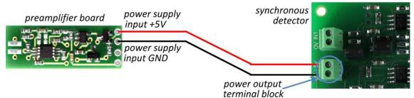
6. Connect the preamplifier output wires to signal input of the PCB-sdetect-3P synchronous detector.
