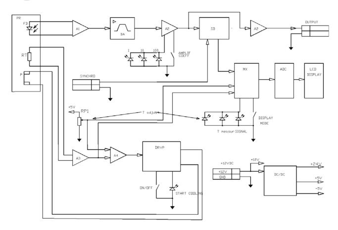
Fig. 12. The Block diagram of AMT-07.
