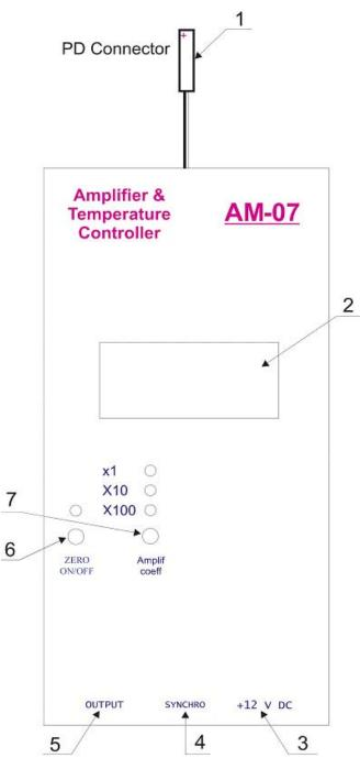
Fig.1. Appearance of the amplifier and its interface.
