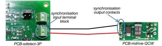
If necessary, make all the connections of other boards (synchronous detector, thermocontroller etc.) following the appropriate instructions manuals. Before turning them on check the required connections and modes:
