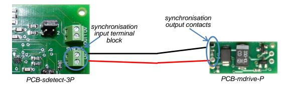
If necessary, make all the connections of other boards (synchronous detector, thermocontroller etc.) following the appropriate instructions manuals. Before turning them on check the required connections and modes:
