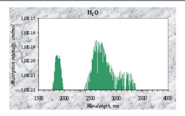
Water has very strong absorption band at 2550-2750 nm and 1830-1900 nm. When applying our LEDs and PDs it is more preferable to use the second absorption band at 1830-1900 nm since emitters and detectors for this spectral range provide much better efficiency.
