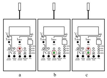
**Fig.11.** a – the LED current is off, b – the Led current is on, c – the LED current is on, but the LED circuit is broken .
