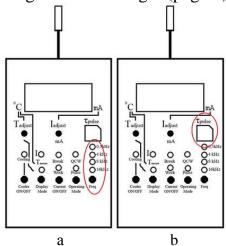
**Fig.10.** a – the button of frequency selection and the indicators of selected frequency, b – the multiposition switch for adjusting the pulse duration.
