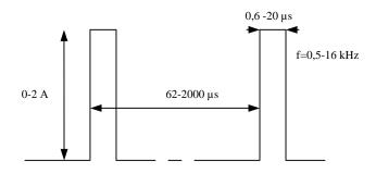
**Fig.2.** Current-time relation in case of pulse mode.
