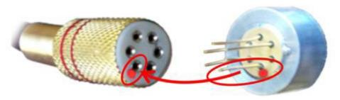
**Fig.4.** Observance of polarity during the connection between the LED and the LED connector (1).
