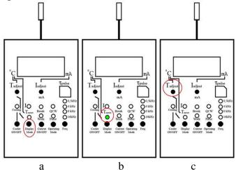
Fig.8. a – the button of display mode selection,
