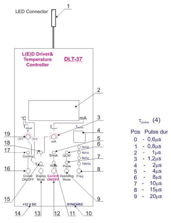
Fig.1. Appearance of the driver and its interface.
