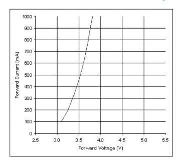
Figure 3. Forward Voltage vs. Drive Current for LXCL-PWF1.
