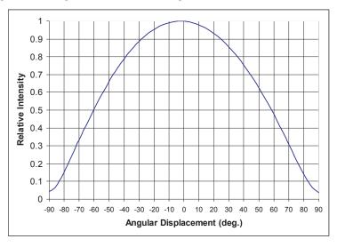
Figure 5. Typical Representative Spatial Radiation Pattern (Far Field) for LXCL-PWF1.
