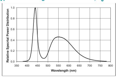
Figure 4. White Color Spectrum of Typical CCT Part, Integrated Measurement.
