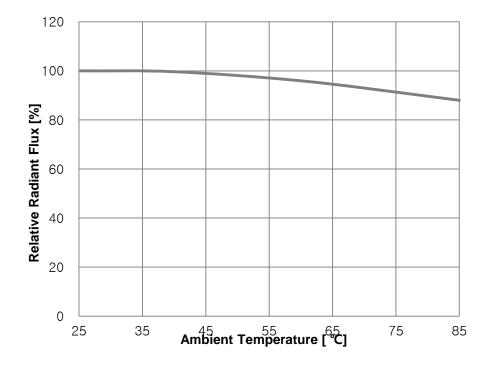
Fig 5. Ambient Temperature vs. Relative Radiant Flux, I<sub>F</sub>=500mA
