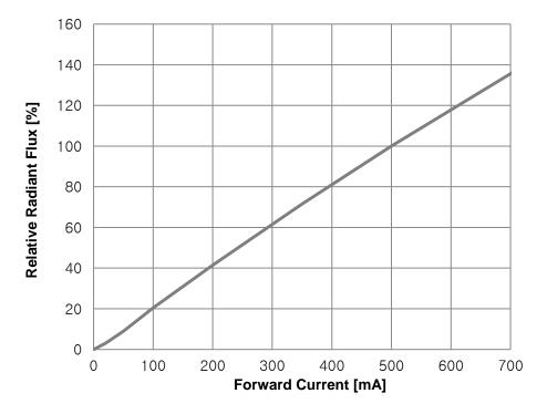
Fig 3. Forward Current vs. Relative Radiant Flux, T<sub>a</sub>=25°C
