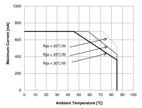
Fig 9. Maximum Forward Current vs. Ambient Temperature, Tj<sub>max</sub> = 125°C
