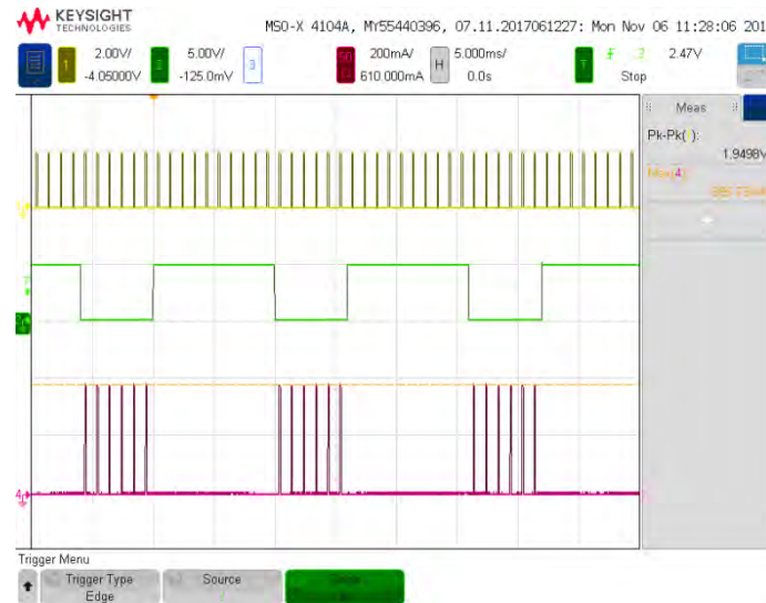
Fig. 12: Burst operation; yellow/upper trace: Input voltage CA-DCSP; green/medium trace: Input voltage CD-ENABLE; red/lower trace: Output current
