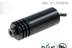
**RLDH980** series of Diode Laser Modules has been designed as a small housing laser module solution. The modules body is made of black anodized aluminum, enclosing laser diode, lens, and driving electronics. RLDH980 series features a *focusable glass lens optic* with a locking mechanism and *incorporated 3 VDC driver* circuit.
