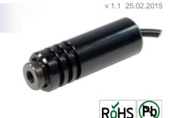
**C2021** series of Diode Laser Modules has been designed with emphasis on *superior beam quality*, and *reliable operation*. The modules body is made of black anodized aluminum, enclosing laser diode, lens, and driving electronics. C2021 series features a *focusable glass lens optic* with a locking mechanism. The supply voltage is specified with *3 VDC*.
